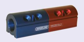
SWAP Valves reduce time required for cooling line evacuation between mold changes to seconds instead of minutes while keeping shop floors clean. SWAP valves use shop air to evacuate fluid from cooling lines with a single handle motion. The mold can then be changed. Resume main cooling fluid supply with the reverse handle motion.
